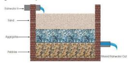
**Pits:** Recharge pits are constructed for recharging the shallow aquifer. These are constructed 1 to 2 m, wide and to 3 m. deep which are back filled with boulders, gravels, coarse sand.
